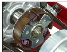
A reliable, centrifugal clutch slips when a buried object is encountered or the auger is overloaded. This protects the flexible drive cable and the transmission gears and shafts from damage.
