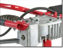
We build our own heavy-duty transmissions that feature cooling fins for quick heat dissipation, o-ring seals, and heattreated shafts and bearings mounted in an oil bath.
