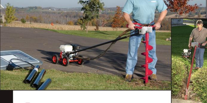
or over 40 years, the versatile Little Beaver mechanical earth drill has been the #1 choice of rental store owners, fencing contractors, and other professionals who require a one-man auger that is safe and simple to operate. Thanks to our patented torque tube, we've eliminated the kickback found in competitive augers, making one-man drilling safe and productive.
