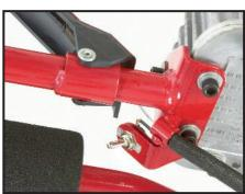
The engine throttle control and the on/off switch are conveniently located on the left handle. Padded handles are ergonomically designed for less fatiguing operation.
