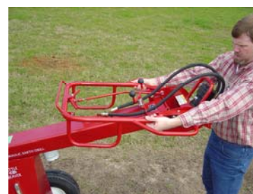
10 Fold handle to rear, remove auger & pull drive head handle forward to lock.
