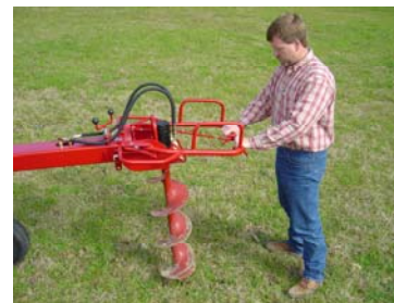
6 Stand clear—pull with right hand to drill. Start auger angled away from engine. Handle may be repositioned as needed to ease control (stop to adjust).
