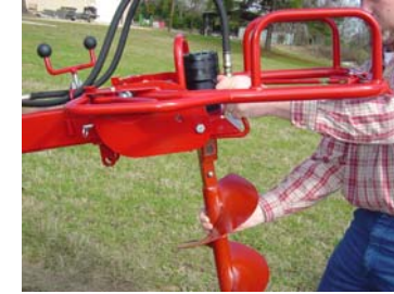
3 Release latch & attach auger. (Machine may be moved w/ auger attached & locked.) Move into position & adjust side-to-side position if necessary.
