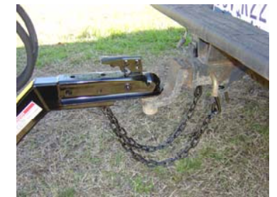
12 Secure to 2" ball. Attach chains. Turn fuel valve off for transporting. Be sure engine fuel valve is in the OFF position.
