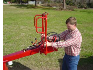
2 Fold handle into operating position. Machine can also be operated with handle in the rearward position for drilling next to a wall.
