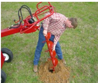
9 Attach extension if necessary to drill deeper (1 max.) Must compensate for arc (push machine back) while drilling.
