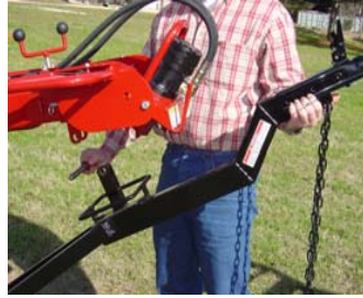
1 Unhook tow bar from 2" ball (vehicle). Remove tow bar from machine.
