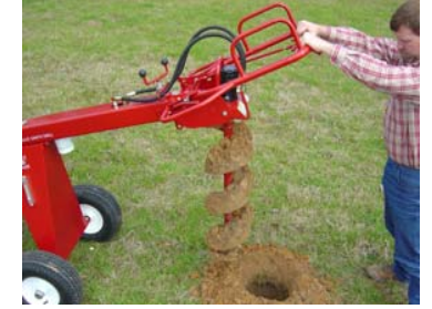
8 Stop auger from turning and pull out when clear.
