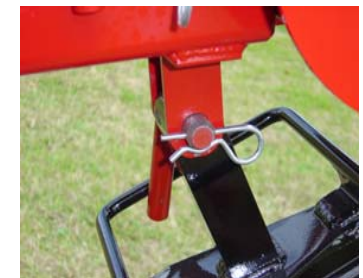
11 Attach tow bar by slipping under reservoir and lifting over hooks. Lift up, attach pin & secure with clip.
