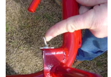
4 Be sure that: The stop switch on the handle is ON. The stop switch on the engine is ON. The engine fuel valve is ON.
