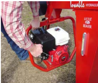
5 Start engine and allow to warm up. Set engine speed control to high speed position.
